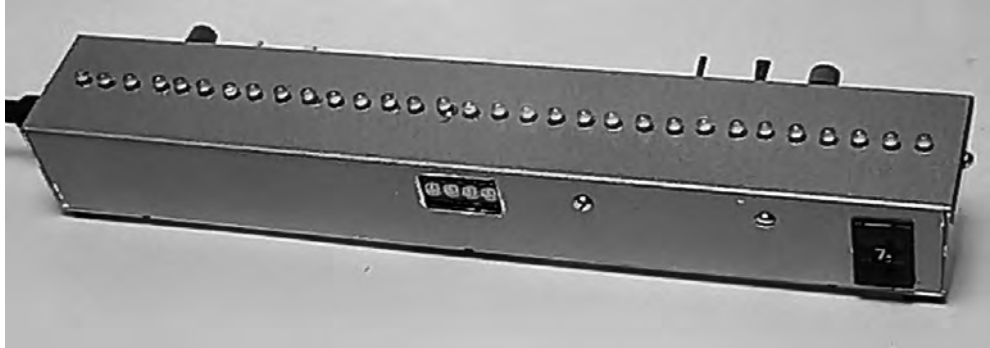
Figure 1. An electronic Random Number Generator built by German Physicist Dr. Helmut Schmidt (1928–2011). An array of 31 LED lamps on the upper face of a parallelepiped metal case featuring a digital display and a mode-regulating counter on its front face.
